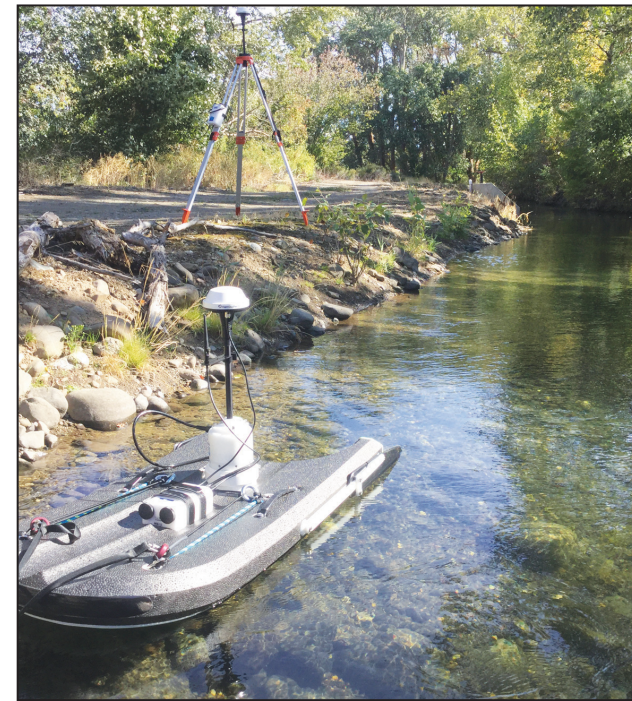
The hydroboard allows for faster and more accurate measurements of flow in canals and creeks.
