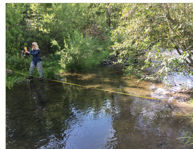
Flow Monitoring: Sherry Swanson (KCCD) measuring stream flow to help with design of a project to improve fish passage.
